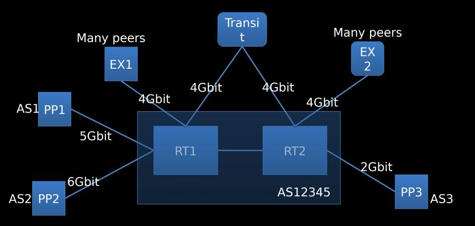
is your largest flow - via PP2 - maybe needs a second private peer backup on P AS1 via PP1, configure a backup over EX1 or EX2 for deterministic rout Can you move larger peers behind EX1 and EX2 onto private peer n exchange failure, where will the traffic go? How big a flow should you care about If you lose RT2, how will traffic to PP3 and traffic volume via EX2 be deliver If you lose RT1, how will traffic volume via PP3 and EX1 be deliver
