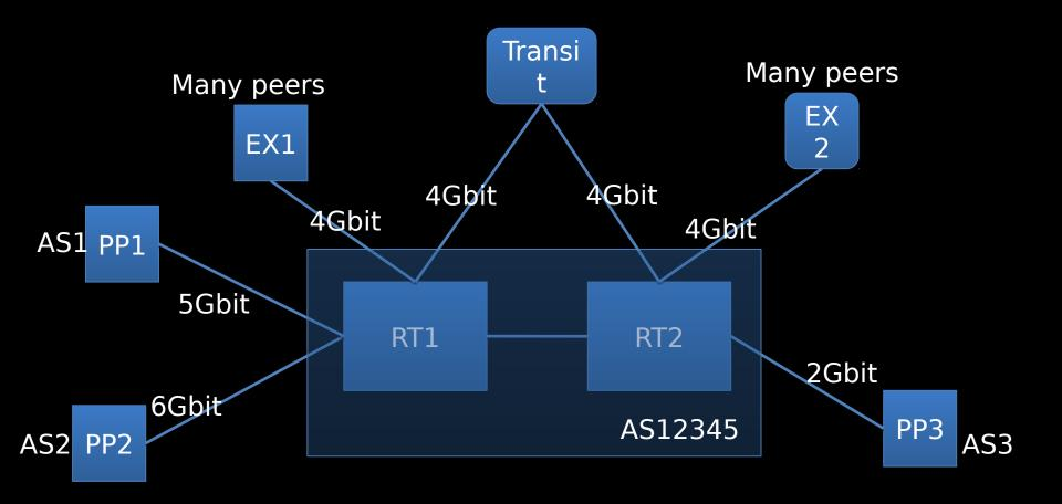
AS2 is your largest flow - via PP2 - maybe needs a second private peer backup AS1 via PP1, configure a backup over EX1 or EX2 for deterministic Can you move larger peers behind EX1 and EX2 onto private p is an exchange failure, where will the traffic go? How big a flow should you care
