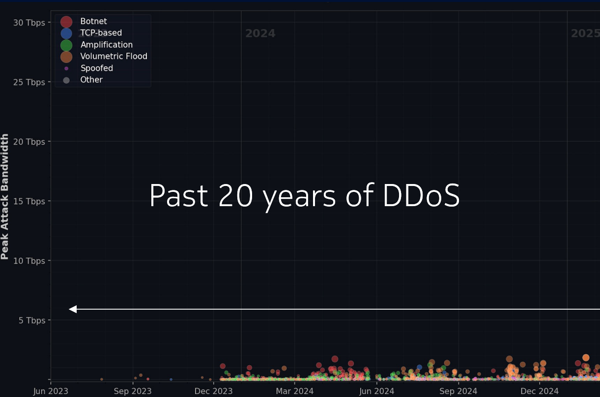
Sample of attacks over last 12 months. Each circle represents individual attack with color (e.g. red == botnet) mapping to attack type and size of circle correlates to duration. DDoS transition from enterprise botnet to Resproxy August 2025
